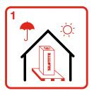
Store Silotite in original protective carton. Store reels on their ends in a dry place out of direct sunlight. The ideal storage temperature is 20
