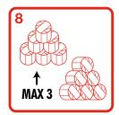
Choose a well drained site away from hedges, trees, exposed areas and water courses. Stack bales immediately after wrapping and within 12 hours. Use a purpose built-handler and never a spike. Do not stack more than 3 high. Bales of low DM should only be stored in single layers. Repair any damage immediately.
