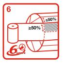
Apply at least a 50% overlap with a minimum 4 layers of film to all areas. For an optimum silage result we advise the application of 6 layers of balewrap. Where DM levels are lower than 30% or are exceeding 50%; for round bales with diameters > 1.3m: for lucerne and for stemmy crops or for square bales, a minimum of 6 layers of film should be applied.
