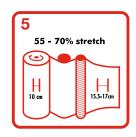
Final width of film as measured on the flat end of a round bale should. with 500mm film be 380mm-420mm. and with 750mm film be 580mm-620mm. Should film width vary outside these limits, stop wrapping and ascertain cause. Ensure prestretch unit rollers are regularly cleaned in accordance with wrapper manufacturer's instructions.
